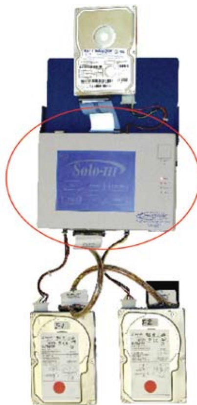
Pic 2: Hardware based hard disk imager (red oval) such as (Masster Solo III) is able to produce two bit-to-bit image copies or two clone copies of the suspect hard disk at time.
