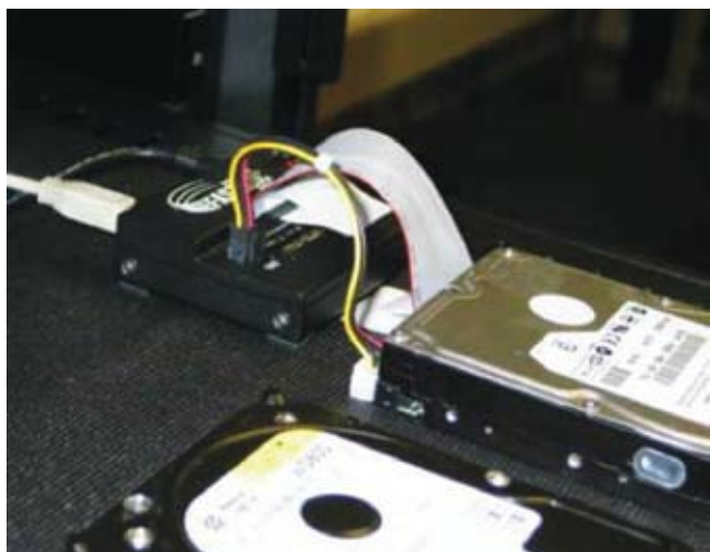
Pic 1: The usage of write blocker (Red oval) will block any writing command to any digital media. It will avoid any tempering on digital evidence, if the exploring and verifying the existence of digital evidence is mandatory, prior to the exhibit collection.
