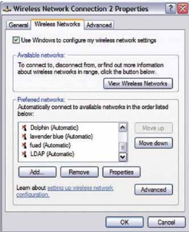
Figure 1: Preferred Network List (PNL) under Windows Zero Configuration (WZC)
