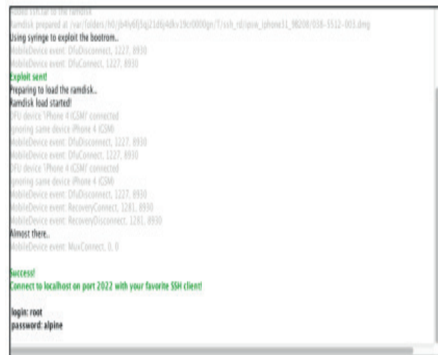
Figure 3: Access to iDevice using SSH.
