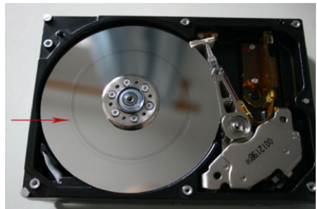
Figure 1 Scratched Hard Disk
