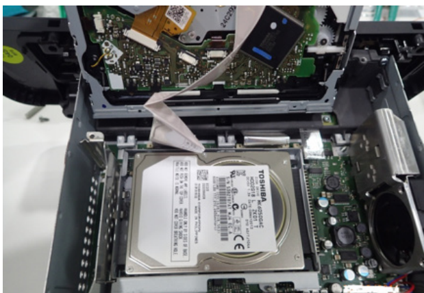
Figure 7: Hard disk inside the infotainment system
