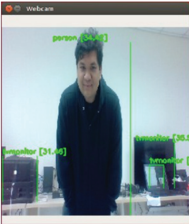
Figure 6: Example of object detection using YOLO
