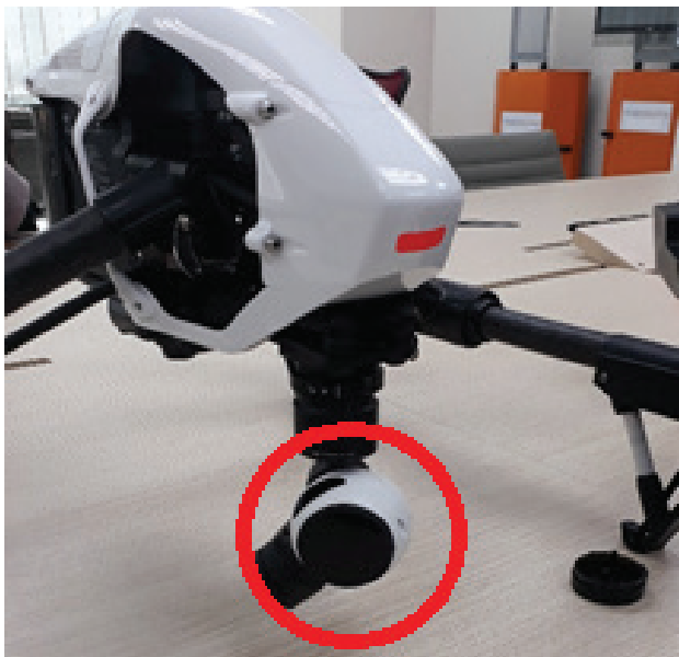
Figure 3: In DJI Inspire 1 the external storage is located at the camera
