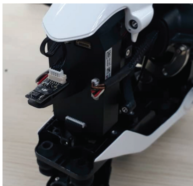
Figure 2: Location of internal storage in DJI Inspire 1
