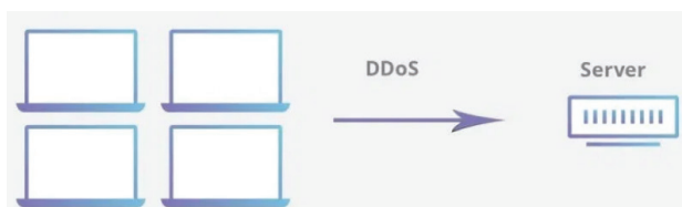
DDoS: Attack from multiple hosts flooding the targeted host
