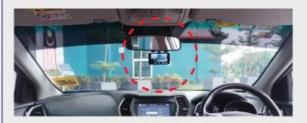
3 THE SUGGESTED ANGLE of view is about 95 degrees facing the front side. Users can adjust viewing angle according to their preferences to provide clear view or playback.
